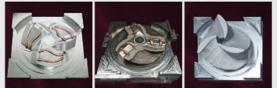
Hexahedron structure build-up by Hybrid-DMT using a metal block (Material : SUS 420J2)
